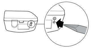
Without turning on the battery, the handset cannot be charged or operate.
