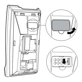
2. Tapping the handset power tact-switch to the off position. When the telephone base and handset successfully enters the energy-saving charging mode, all keys on the telephone base should not respond.
