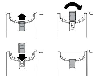
Install the telephone base as shown.
