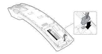
4. To replace the handset cover, align all the tabs on the handset cover against the corresponding grooves on the handset, then firmly push downward until all the tabs lock in the grooves. Then install the screw.
